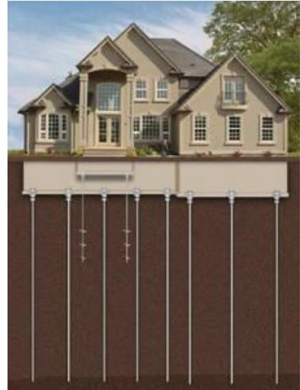
Underpinning with helical piers is accomplished by extending the foundation in depth or width so it either rests on a more supportive soil stratum or distributes its load across a greater area. Use of steel piers, helical anchors and micropiles are the most common methods in underpinning.
