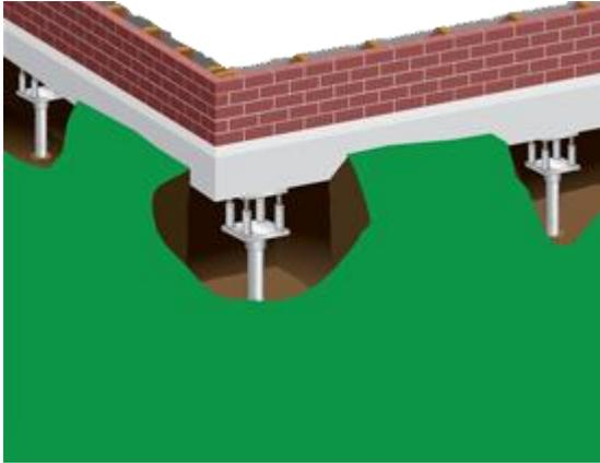
**7. Restoration:** Under careful supervision, the load is transferred from the failing soil under the foundation to the pier system. The structure is gently and evenly lifted to as close to the original elevation as the structure will allow or to the specified design elevation. The adjustment rods are tightened on the bearing plate the pier caps are secured at each placement and the lifting equipment is removed.
