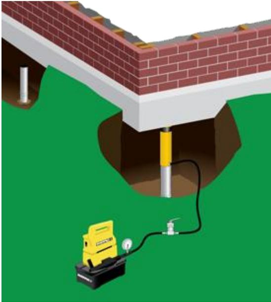
**4. Pier Pipe Installation:** The pier pipe is advanced into the soil using a small portable high-pressure hydraulic cylinder and pump. Each section of pier pipe measures 12” long so low overhead clearance is not a problem during installation. The piers may be installed from outside or inside the structure.
