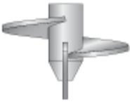
ECP HD Extreme Anchors give users high-strength anchor capability in rocky and debris laden soils. These 10,000 lb. and 15,000 lb. capacity anchors have 2-1/4" and 2-1/2" hubs, respectively. ECP Utility's unique beveled cutting edge allows the 1/2" helix to power through the toughest soil conditions.
