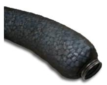
EZflow is a gravel-free alternative to a traditional French Drain system. Each EZflow section contains a 10 foot-long plastic corrugated pipe surrounded by EZflow Poly Rock aggregate structurally engineered to have an increased void space. Pipe and aggregate are enclosed in a strong and durable mesh material to prevent clogging.
