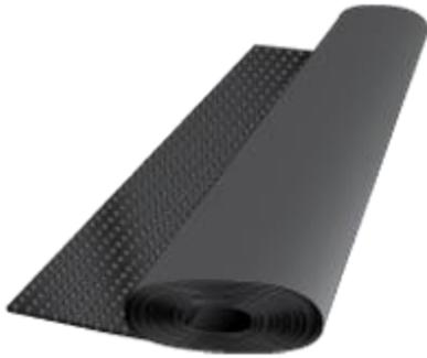
Sheet Drains for single side drainage applications are prefabricated products that consist of a solid, formed, three dimensional core covered with a geo-textile filter fabric bonded to the dimple side of the core.
