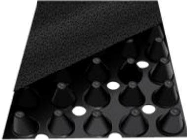
ECP Strip Drains are prefabricated drains that consist of a high-profile, perforated, three-dimensional core (6" high x 1" wide x 150' long) that is fully wrapped with a filter fabric.
