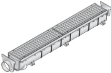
The ECP Channel Drain is a lightweight drain system with interlocking joints, so connections are made quickly and easily. The modular design offers flexibility as each 40" section of channel can be snapped together for longer runs or divided down to lengths as short as 4" for smaller, interlocking sections.
