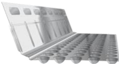
The ECP Water channel is an interior basement floor drainage system for new construction and retrofitting. Engineered to sit on top of the footing to create a pathway for water to flow from the wall and cold joint, across the footing and into the drain system. This unique design provides added strength to the channel to prevent collapsing and warping along the wall and creates a thermal break between the footing and slab.
