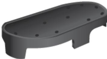
**The BSPS pump stand** is a rigid base that provides a platform for sump pumps, keeping them away from sump pit debris. By insuring that the sump pump does not pickup debris off the bottom of sump basins, sump pump impellers and check vales will last longer.
