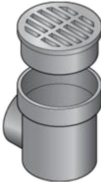
ECP offers round catch basin and grates that can be used for downspout and sump pump discharge. As hydro-static pressure builds in the drain pipe, water will seep out the top of the grate to a suitable drainage area or storm drain.
