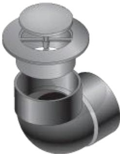
The ECP Pop-Up Emitter provides a cost effective, yet esthetically pleasing, way to provide downspout and sump pump discharge away from foundations. ECP Pop-up Emitters are designed to rise above grade when water is present and then they are spring loaded to retract to allow for easy mowing. This simple system will provide years of maintenance free use while protecting your basement walls from hydrostatic pressure caused by excessive water in the soil.
